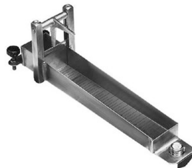
29.12 Photo of Bostwick consistometer (Courtesy of Cole-Parmer, Vernon Hills, IL) figure
