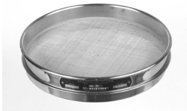
34.1 figure Fisher US standard test sieve. Range of mesh sizes is available for various particle size separations
