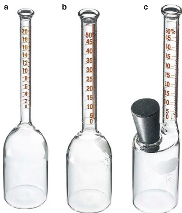
17.5 Babcock milk test bottles for milk (a), cream (b), and cheese (Paley bottle) (c) testing figure (Courtesy of Kimble Glass Co., Vineland, NJ)
