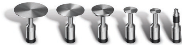
29.15 Photos of cone and plate and parallel plate test fixtures for rheological measurements (Courtesy of TA Instruments, New Castle, DE)
