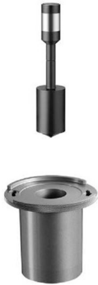
29.10 Photo of cup and bob test fixtures (concentric cylinder geometry) for rheological measurements (Courtesy of TA Instruments, New Castle, DE) figure
