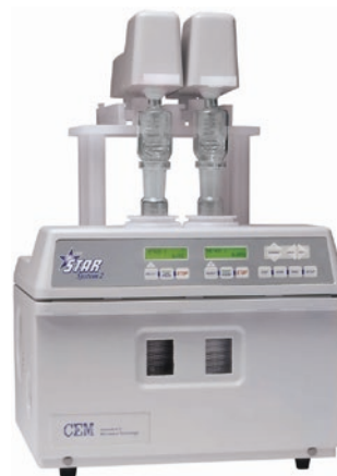
16.2 figure Microwave open-vessel system (Courtesy of CEM Corporation, Matthews, NC)
