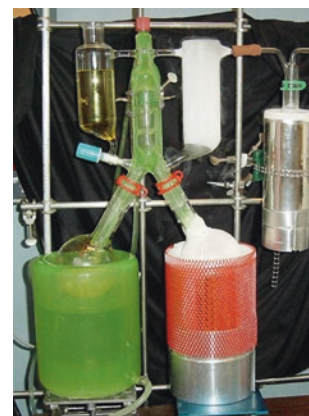
14.3 figure Solvent-assisted flavor evaporation (SAFE) distillation system
