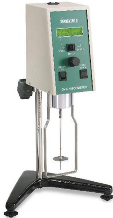
29.11 Photo of Brookfield viscometer (Courtesy of Brookfield AMETEK, Middleboro, MA) figure
