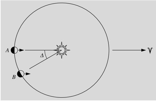
**Fig. 2.31** One sidereal day is the time between two successive transits or upper culminations of the vernal equinox. By the time the Earth has moved from  $A$  to  $B$ , one sidereal day has elapsed. The angle  $\Delta$  is greatly exaggerated; in reality, it is slightly less than one degree
