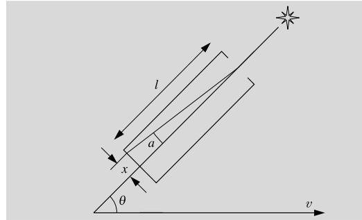
**Fig. 2.21** A telescope is pointed in the true direction of a star. It takes a time  $t = l/c$  for the light to travel the length of the telescope. The telescope is moving with velocity  $v$ , which has a component  $v \sin \theta$ , perpendicular to the direction of the light beam. The beam will hit the bottom of the telescope displaced from the optical axis by a distance  $x = tv \sin \theta = l(v/c) \sin \theta$ . Thus the change of direction in radians is  $a = x/l = (v/c) \sin \theta$
