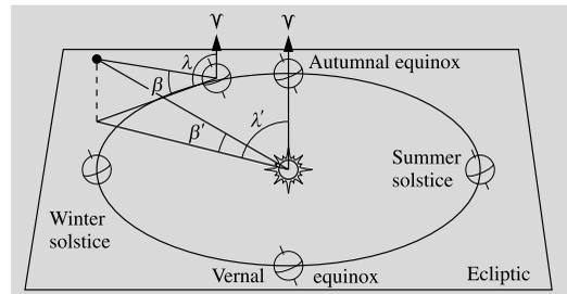
**Fig. 2.15** The ecliptic geocentric ( $\lambda, \beta$ ) and heliocentric ( $\lambda', \beta'$ ) coordinates are equal only if the object is very far away. The geocentric coordinates depend also on the Earth's position in its orbit
