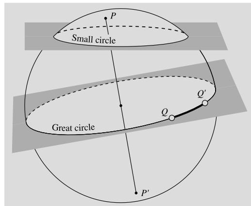
**Fig. 2.1** A great circle is the intersection of a sphere and a plane passing through its centre.  $P$  and  $P'$  are the poles of the great circle. The shortest path from  $Q$  to  $Q'$  follows the great circle
