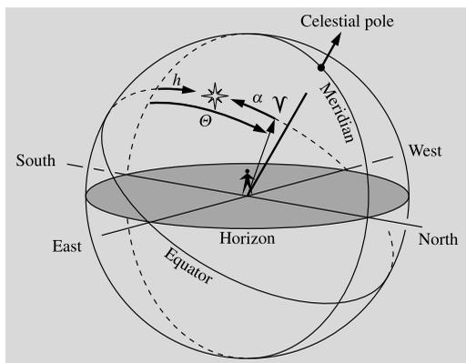
**Fig. 2.11** The relation between the right ascension  $\alpha$ , hour angle  $h$  and sidereal time  $\Theta$ . The right ascension is measured counterclockwise from the vernal equinox, the hour angle and sidereal time clockwise from the South meridian. The sidereal time is the hour angle the vernal equinox
