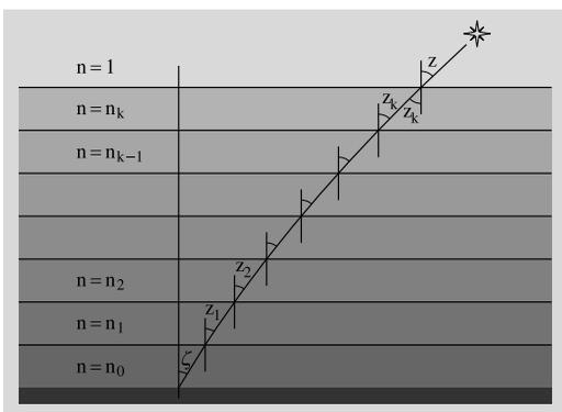
**Fig. 2.22** Refraction of a light ray travelling through the atmosphere. If the altitude is not very low we can think that the atmosphere consists of planar layers each of which has its own index of refraction. Outside the atmosphere the index is  $n = 1$  and increases towards the ground
