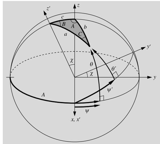
**Fig. 2.6** To derive triangulation formulas for the spherical triangle  $ABC$ , the spherical coordinates  $\psi$ ,  $\theta$ ,  $\psi'$  and  $\theta'$  of the vertex  $C$  are expressed in terms of the sides and angles of the triangle
