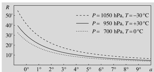
**Fig. 2.23** Refraction at different altitudes. The refraction angle  $R$  tells how much higher the object seems to be compared with its true altitude  $a$ . Refraction depends on the density and thus on the pressure and temperature of the air. The upper curves give the refraction at sea level during rather extreme weather conditions. At the altitude of 2.5 kilometers the average pressure is only 700 hPa, and thus the effect of refraction smaller (lowest curve)
