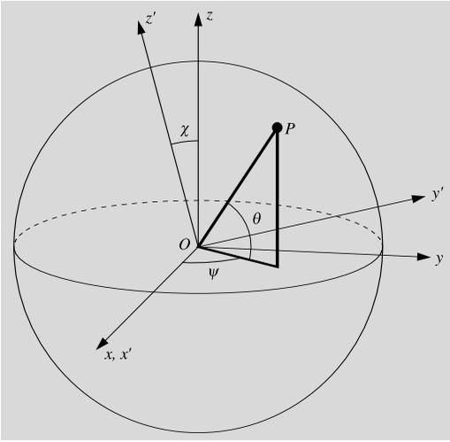
**Fig. 2.4** The location of a point  $P$  on the surface of a unit sphere can be expressed by rectangular  $xyz$  coordinates or by two angles,  $\psi$  and  $\theta$ . The  $x'y'z'$  frame is obtained by rotating the  $xyz$  frame around its  $x$  axis by an angle  $\chi$
