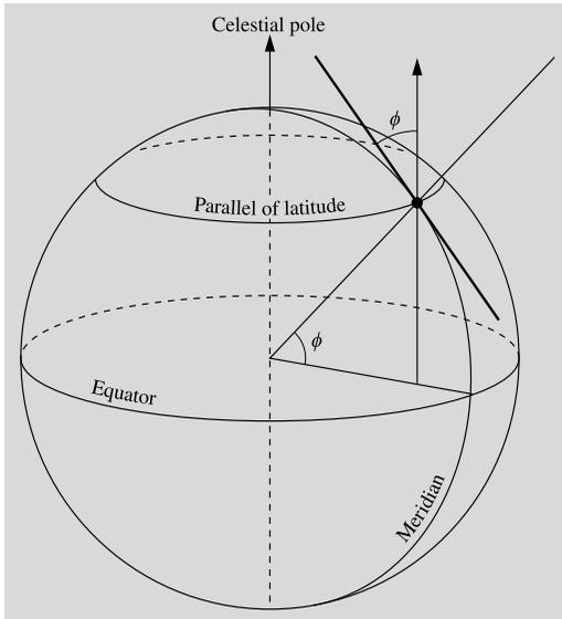
**Fig. 2.7** The latitude  $\phi$  is obtained by measuring the altitude of the celestial pole. The celestial pole can be imagined as a point at an infinite distance in the direction of the Earth's rotation axis
