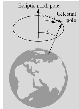
**Fig. 2.18** Due to precession the rotation axis of the Earth turns around the ecliptic north pole. Nutation is the small wobble disturbing the smooth precessional motion. In this figure the magnitude of the nutation is highly exaggerated
