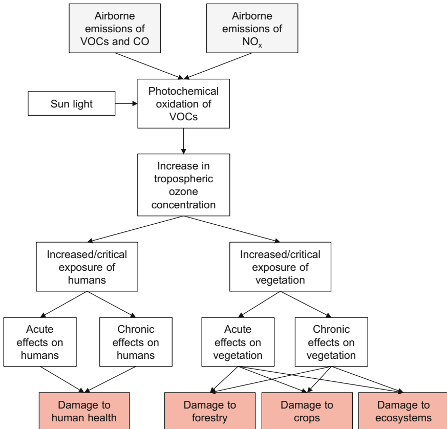
Fig. 10.16 Impact pathway for photochemical ozone formation [adapted from EC-JRC (2011)]
