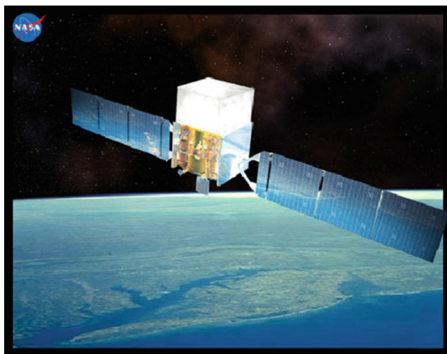
Fig. 1.49 Artist's drawing of the Fermi satellite, launched in 2008. Fermi observes at energies between 10 keV and 300 GeV. Credit: NASA E/PO, Sonoma State University, Aurore Simonnet
